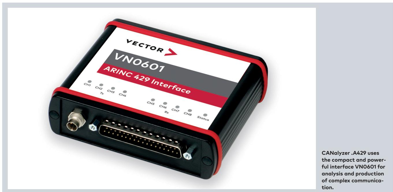
**CANalyzer .A429 uses the compact and powerful interface VN0601 for analysis and production of complex communication.**
