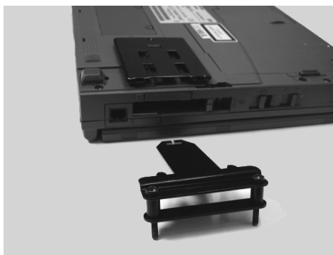
Fig.12: For transportation of the notebook in a bag, unscrew the clamping plate, use a coin like fig.5 and remove the connector fixture.
