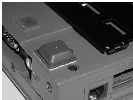
Fig.7: Apply the rubber feet to the bottom of the notebook.
