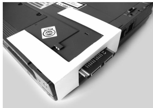
Fig.2: Center the template on the bottom side of the notebook with a partially inserted PC-Card.
