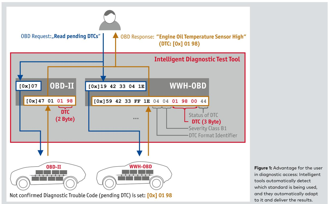
**Figure 1:** Advantage for the user in diagnostic access: Intelligent tools automatically detect which standard is being used, and they automatically adapt to it and deliver the results.
