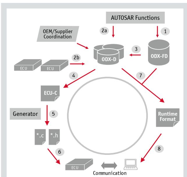
**Figure 4:** Combination of ODX and AUTOSAR
