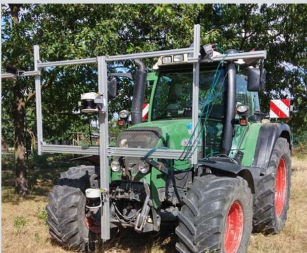
Figure 1: Prototype setup for testing environmental sensors of the slave tractor
