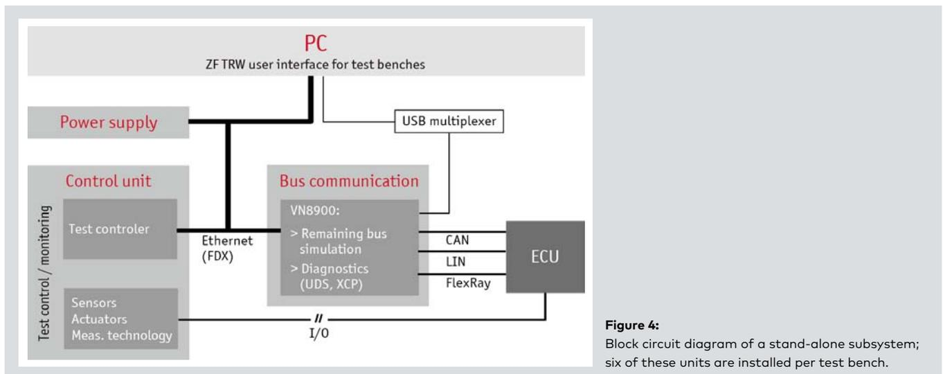
**Figure 4:** Block circuit diagram of a stand-alone subsystem; six of these units are installed per test bench.
