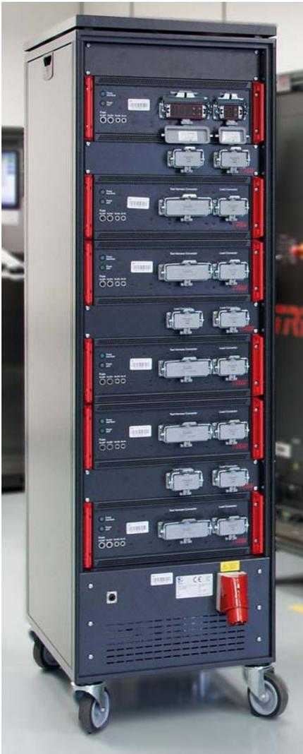
**Figure 1:** Six rack-mounted units or subsystems, each of which represents a unit for testing one ECU. One test bench can test a total of six ECUs simultaneously.
