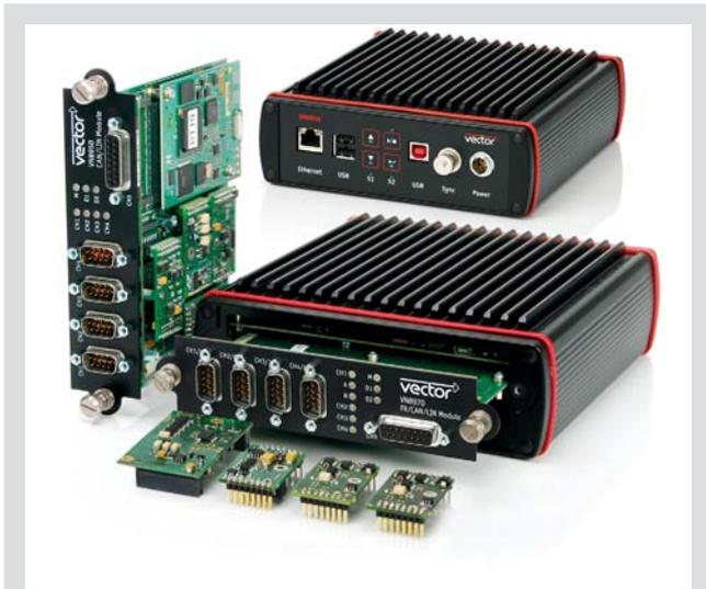
**Figure 3:** The modular VN8900 network interface with integrated real-time computer plays a central role in the ECU's network communication.
