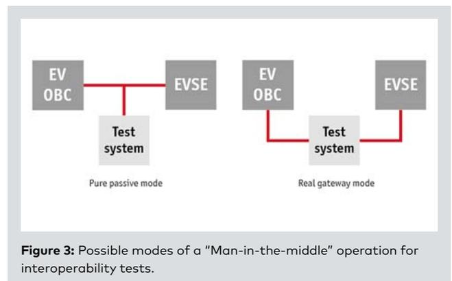
**Figure 3:** Possible modes of a "Man-in-the-middle" operation for interoperability tests.
