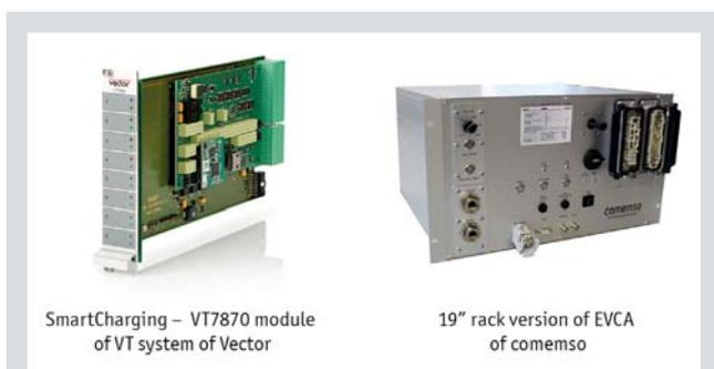
**Figure 5:** Test system components for SCC tests relating to IEC 61851 and IEC/ISO 15118.
