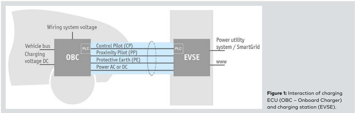
**Figure 1:** Interaction of charging ECU (OBC – Onboard Charger) and charging station (EVSE).
