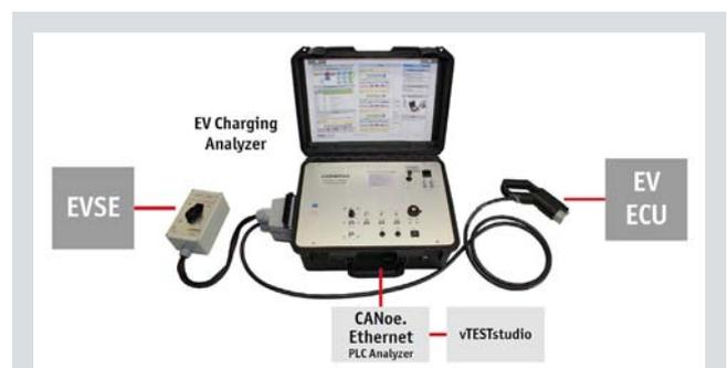
**Figure 6:** Test system combination for mobile use.
