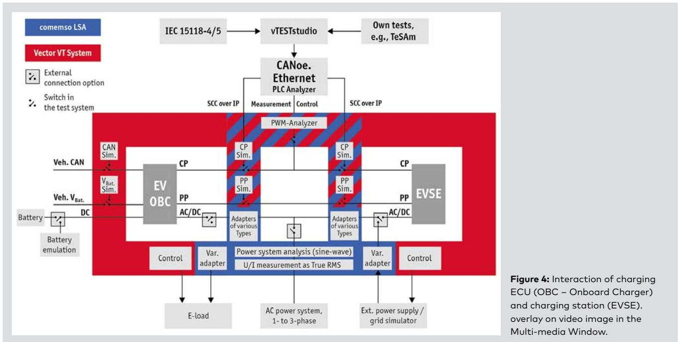
**Figure 4:** Interaction of charging ECU (OBC – Onboard Charger) and charging station (EVSE). overlay on video image in the Multi-media Window.
