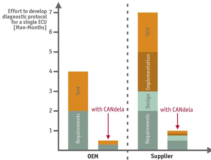
[Figure 4: Cost savings by a factor of 6-7 due to description of diagnostic data using CANdelaStudio and the resulting quicker implementation of the diagnostic protocol]
