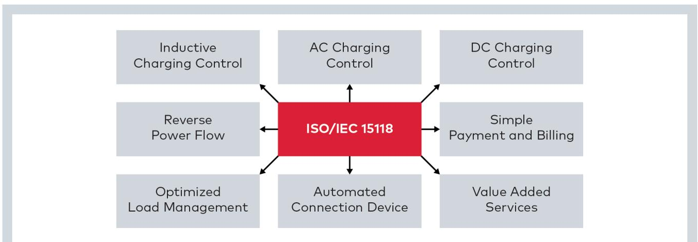
Figure 2: ISO/IEC 15118 is the international standard for charging communications.
