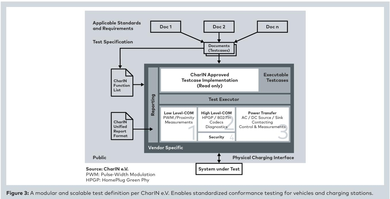
Figure 3: A modular and scalable test definition per CharIN e.V. Enables standardized conformance testing for vehicles and charging stations.
