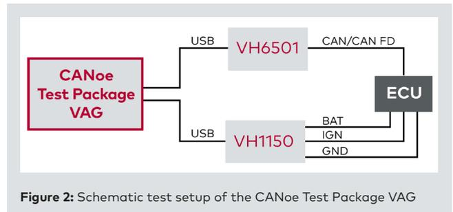
used to simulate digital and analog disturbances on the CAN (FD) network. At the same time, it serves as a normal CAN (FD) network interface. It reproducibly alters the physical properties and the logical levels. Flexible trigger and disturbance logic enables specific corruption of CAN (FD) messages at any bit positions.
