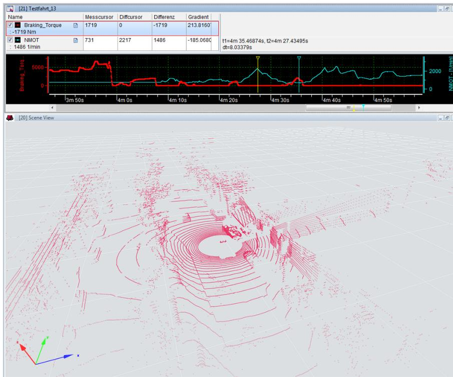
Figure 1: For ADAS development, CANape records LIDAR sensor data from Velodyne, Ibeo and Quanergy and displays this as highly informative point clouds.
