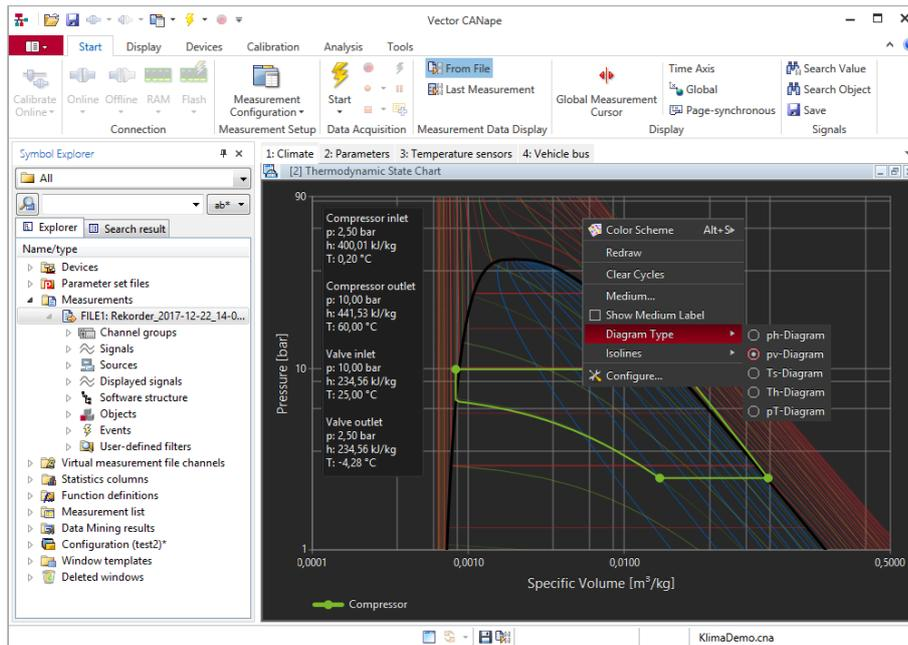
Figure 2: With the option “Thermodynamic State Charts”, air conditioning and cooling system developers can now also display thermodynamic data synchronously with other measurement data and generate state charts for online and offline analysis. Image rights: Vector Informatik GmbH.
